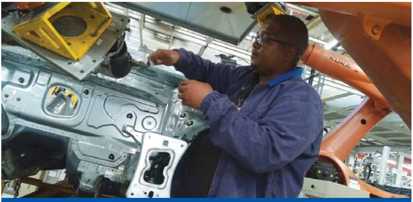
» Smith replacing the collet of the Robot Tucker gun.
