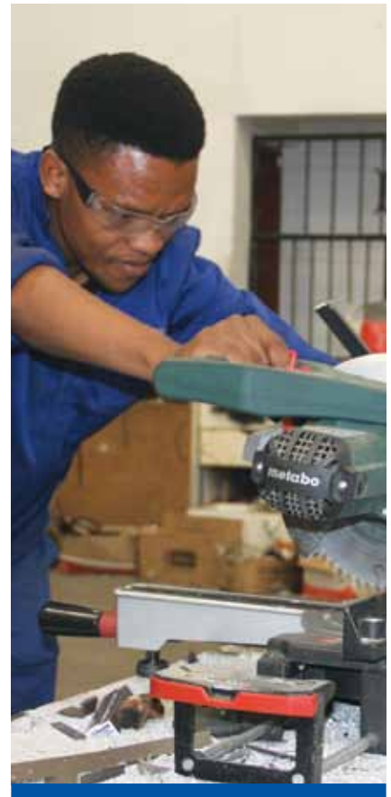
» Madlenkosi Mchunu cutting "beading" for a frame which works to put glasses in position.
