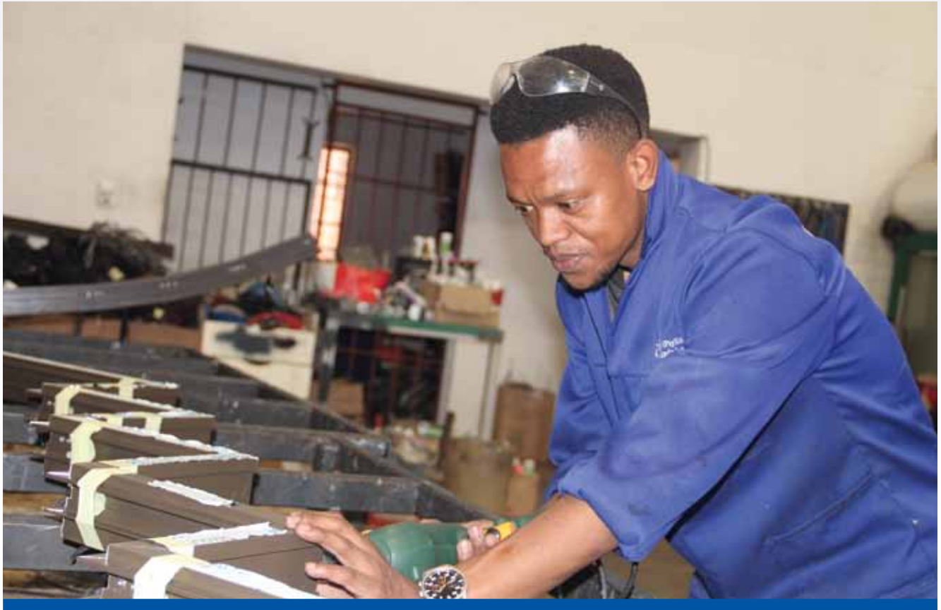
» Madlenkosi Mchunu assembling a frame that will fit onto stairs, closing it off from the space next to it.
